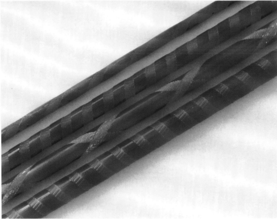
Figure 1. An example of CFRP tension elements fabricated by the pultrusion method.
